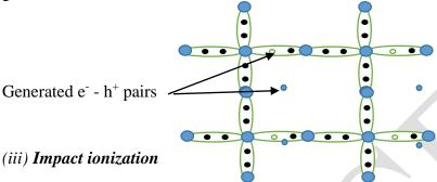
When a semiconductor is under an electric field, one energetic charge carrier will create another charge carrier. For a very high electric field, it results in an avalanche breakdown.
