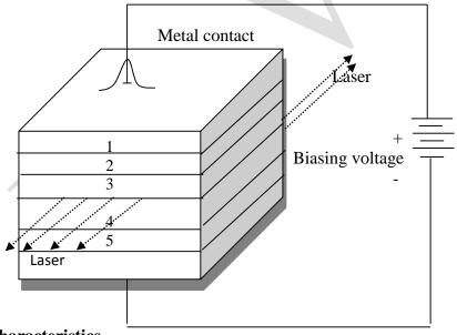
Layer1: GaAs - p type Layer2: GaAs - p type Layer3: GaAs - p type Layer 4: GaAs - n type Layer 5: GaAs - n type
