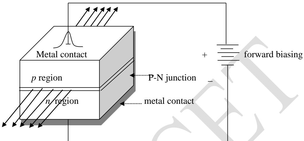
The photon emission is stimulated by a thin layer of PN junction. The potential difference is applied to the homojunction diode through the metal contact .the end faces of the junction are polished and made parallel to each other. They act as optical resonator (the diode has high refractive index) where the laser comes out.
