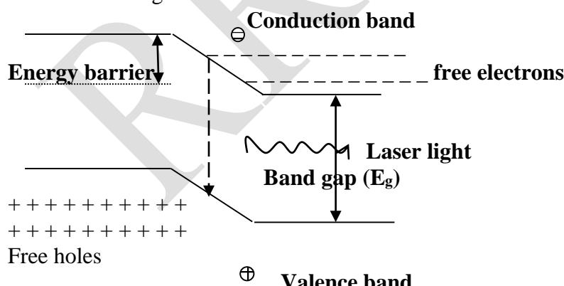
When the forward biased voltage is increases, the emitted photon multiplies and triggers these recombining photons in phase. These photons moving at the plane of junction travels back and forth by reflection between two sides of the junction and grows in strength. After gaining enough strength it emits a laser beam of wavelength  $8400\text{A}^\circ$ . The wavelength of emitted radiation depends on (i) band gap & (ii) the concentration of donor & acceptor atoms. The
