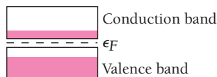
Figure 10.25 The valence and conduction bands in a semiconductor are separated by a smaller gap than in the case of an insulator. Here a small number of electrons near the top of the valence band can acquire enough thermal energy to jump the gap and enter the conduction band. The Fermi energy is therefore in the middle of the gap.
