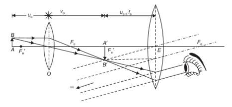
In formula (*ii*) and (*iii*) we shall substitute only the numerical values of vo, uo, fe and D. Negative sign shows that the final image is inverted. It is clear from these formula that in order to increase the magnifying power of microscope:
