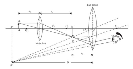
**Magnifying Power:** Suppose the final image A"B" subtends an angle  $\beta$ at the eye-piece E. Since eye is very near to the eye-piece, the angle  $\beta$ can also be taken as subtended by A"B" at the eye. Suppose when the object AB is at the least distance of distinct vision D, then it subtends an angle  $\alpha$  at the eye. The magnifying power of the microscope is
