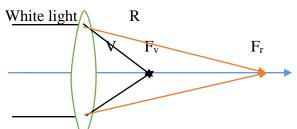
A beam of white light is incident on a convex lens parallel to principal axis. The dispersion of colours takes place due to prismatic action of light. Violet is deviated most and red as least. Red is brought to focus at a point farther than the violet. Hence The difference  $f_v - f_r$  is a measure of the axial chromatic aberration of a lens for parallel rays.
