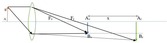
Figure shows a convex lens and n object placed in front of the lens. The lens forms the image of white object AB as  $B_v A_v$  and  $B_r A_r$  in violet and red colours respectively. The images on other colours lie in between the two. Evidently the size of red image is greater than the size of the violet image. The difference is a measure of lateral chromatic aberration.
