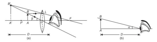
In Figure (a), AB is a small object placed between a lens L and its first focus F'. Its magnified virtual image A'B' is formed at distance D from the lens, the distance of the image A'B' from the eye is also D.
