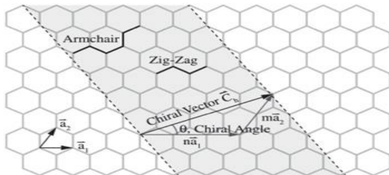
Figure 1. Schematic representation of rolling graphene layer to create CNT 15 .
