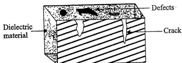
Fig. 5.13. Defects and Cracks in Dielectric Material
