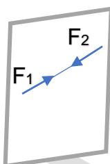
**Coplanar concurrent forces:** Forces intersects at a common point and lies in a single plane.
