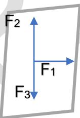
**Coplanar non-concurrent forces:** Forces which do not intersect at a common point, but acts in a single plane
